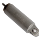
Exhauster Brake Cylinders
